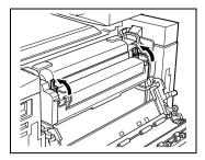
6 Move the levers (one on each end of the oil-coating unit) in the direction of the arrows and carefully pull out the paper.
